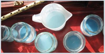
Levigation is the process which separates the different sizes of particles in water. The smaller and lighter weight particles float at the top of the water and take longer to settle. The smaller particles are also lighter in colour.
